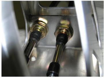
To mount the nuts take off the rubber boot, then the nuts can be mounted easily
