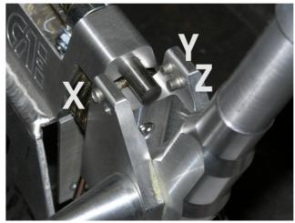
Now select gear 5 with the gearshift and turn stop screw X until the 5th gear can be selected clearly. Press rear stop bolt and enter rear gear. Turn stop screw Y until the rear gear can be selected clearly.
