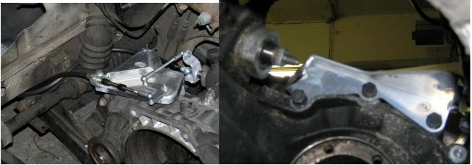
Mount connecting Rod "S" on the gear unit entry lever (Picture shows the old Version)
