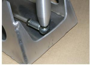
Secure the seats on the cables in the selector-tower. Select level 1 / 2 with gearshift and turn stop screw Z until the gears 1 and 2 can be selected well.
