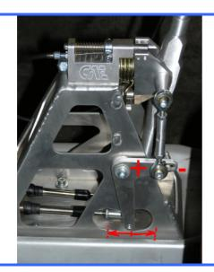
The selection-way of the gearshift is adjustable by changing the position of the lower ball joint. This can be necessary, if not all gears can be achieved (selection-way too much) or the levels of the gears are to close to each other. (selection-way too small) The bell crank should be placed in the 3rd /4th gear (middle position) like shown in the picture.
