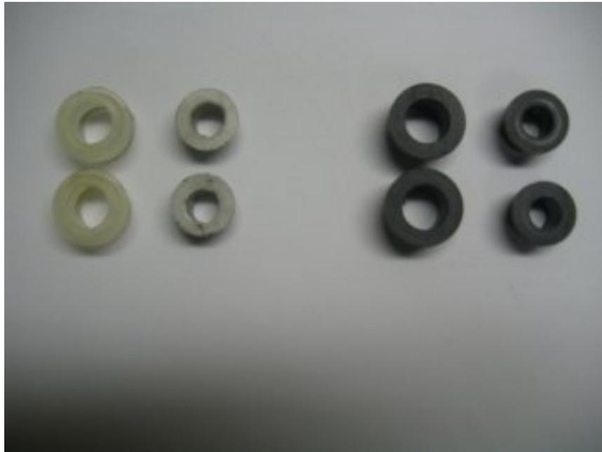
Pictured on the left are the factory pivot bushings. The large ones are found on the relay shaft, the small ones are located on the pivot bolted to the transmission itself. These are replaced with solid Delrin® equivalences.
