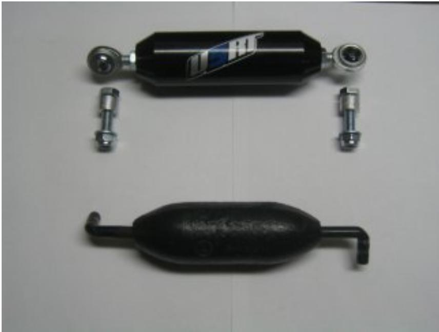
This is the weighted rod. MK3 drivers will notice the stock weighted piece, which is interchangeable with the MK2 non-weighted link. Rabbit & Scirocco owners have a similar link to the factory MK2 link. The factory link can be removed entirely. The new link is provided with two long bolts and lock nuts, as well as a washer and two press-in spacers.
