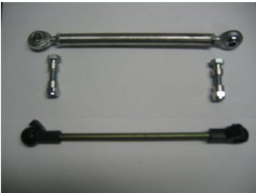
This is the long link that goes between the two shift levers. It can be removed entirely, and is replaced with a solid aluminum link. The bolts should be installed by having a bushing on either side of the heim joint.
