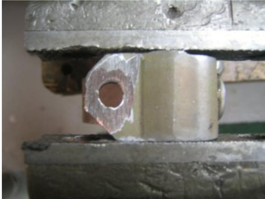
Once the stud is removed, it is highly advisable to ream the hole with a 5/16" drill bit. This process needs to be followed for all of the ball-joints that the heim joints replace
