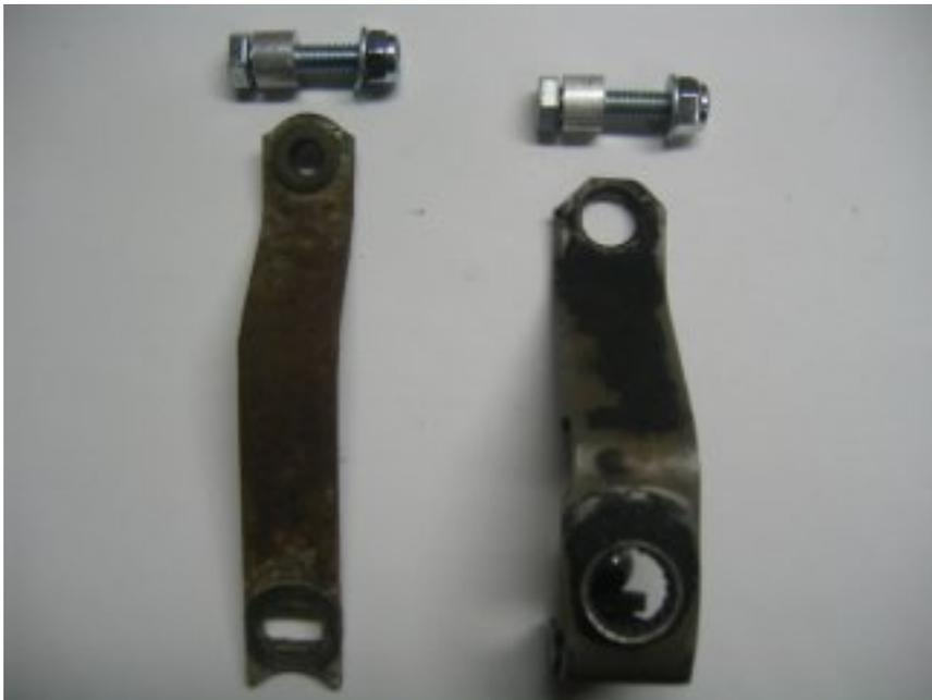
These are the two shift levers. On the ends of these levers are two rubber grommets. These grommets need to be removed entirely. The two press-in spacers found on the long bolts will be pressed into the holes. It should be pressed flush on one side, and should protrude on the side that has the heim joint of the weighted rod. On the opposing side of the heim, install the washer, and tighten the lock-nut firmly in place.
