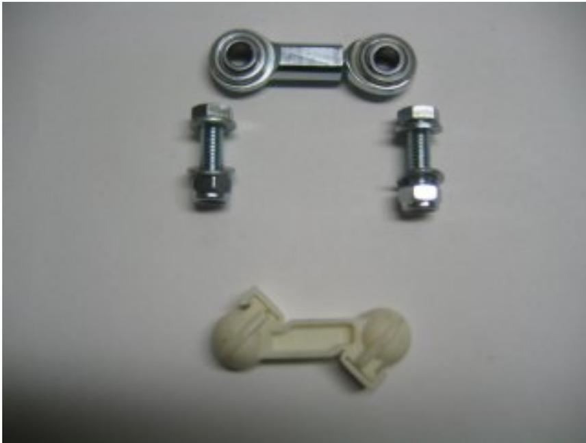
The lower piece will be found on all generation chassis. On the A1, it is slightly longer. This is the piece that goes between the lever on the transmission, and the pivot mechanism on the transmission. A1 kit owners will be provided with a complete aluminum link. This piece requires that the factory lever and transmission mount are modified. Installation should have a washer on either side of the heim joint.
